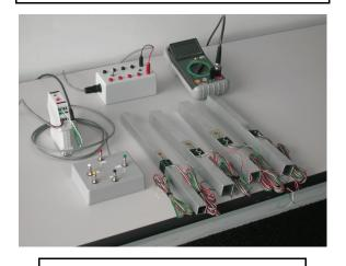
Wire full bridges to measure axial, torsion, transverse shear, and bending loads.
