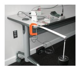
Calibrate a cantilever beam weigh scale and calculate shunt cal resistor equivalent force as well as mV/V output.
