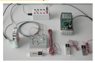
Investigate Wheatstone Bridge behavior, thermal compensation, lead wire effects, and shunt calibrations.
