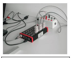
Workshops incorporate commercial data acquisition systems for exposure to real world instrumentation. Mars Labs and HBK equipment
