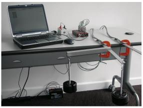
Measure rosette strain gage responses from beams under combined loads and calculate the resulting multiaxial stresses.
