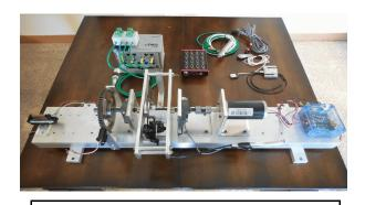
This small motor dynamometer is used as a data acquisition platform for students to connect sensors to different data acquisition systems and record and analyze results in real time.
